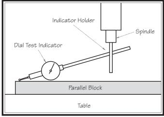
Figure 28. Dial test indicator mounted.
